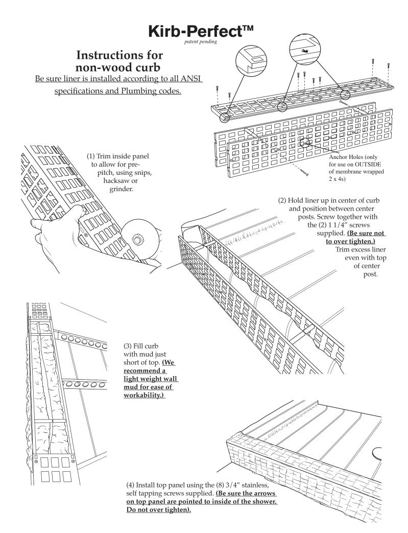
(5) Fill balance of curb with mud and screed top and sides.
